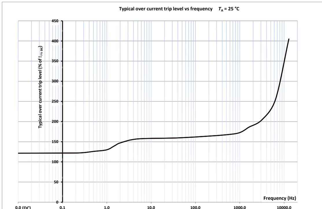
The table shown below summarizes various frequency values and the typical value of over current trip level to detect over current state:
