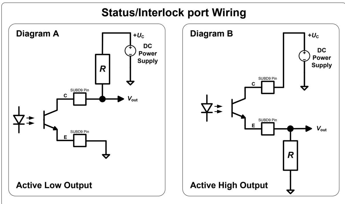
In the Diagram A Active Low Output, the output signal  $V_{out}$  switches to GND when the corresponding LED is ON.
