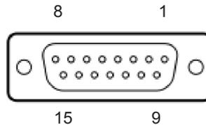
The pins 1 to 3 are internally shorted by rack electronics. It is the same for pins 9 to 11.
