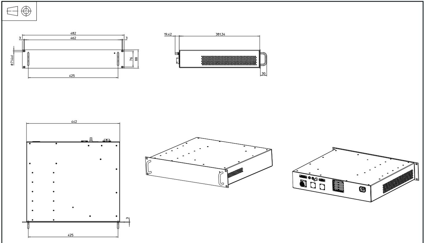
**Dimensions - ITZ 2000 measuring head (in mm)**
