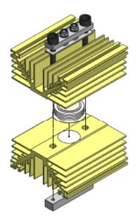
Clamps with dual force indicators must be tightened evenly. The belleville washers under both indicators must turn freely for correct installation.
