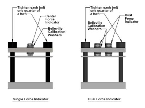
Darrah Electric's semiconductor mounting clamp uses a two bolt system with a pre-calibrated center force indicator. The correct force is achieved when the belleville washers located under the center force indicators are free to spin. Lighter clamp force requires only a single force indicator, higher clamp forces require dual indicators. These pre calibrated force indicators eliminate any need for special gauges or torque wrenches.
