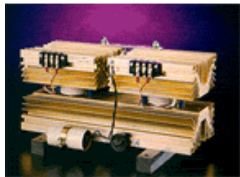
Fig. 3 - Fins add surface area to help convect heat away from the natural convection - cooled SCR contactor.
