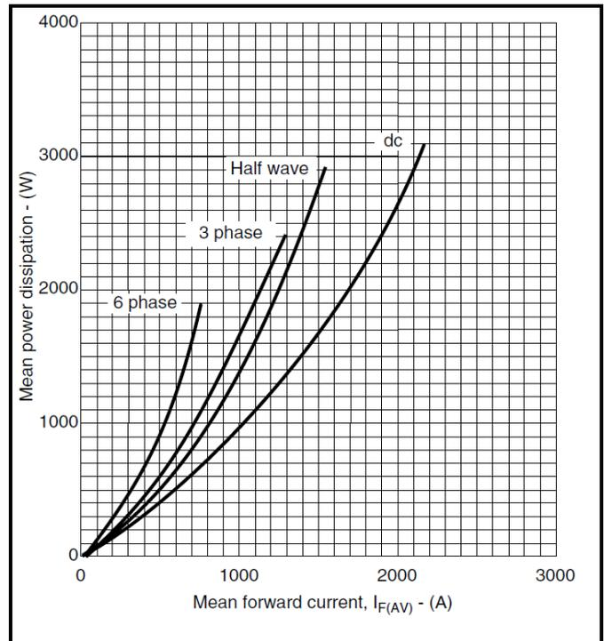
Fig.3 Dissipation curves
