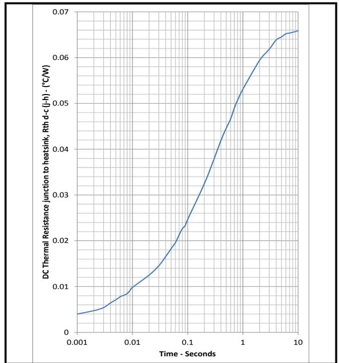
Fig.7 Maximum (limit) transient thermal impedance-junction to heatsink
