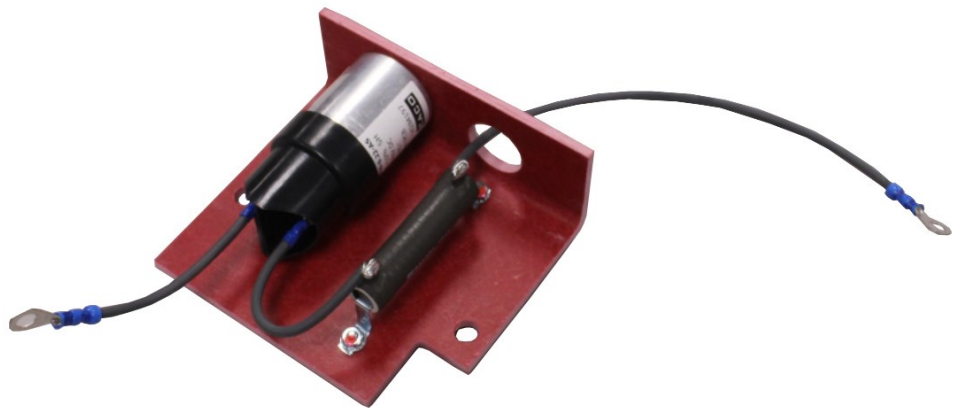
New R/C Snubber Higher Voltage Capacitor, Non-Inductive Resistor. 2KV Insulated Wire.
